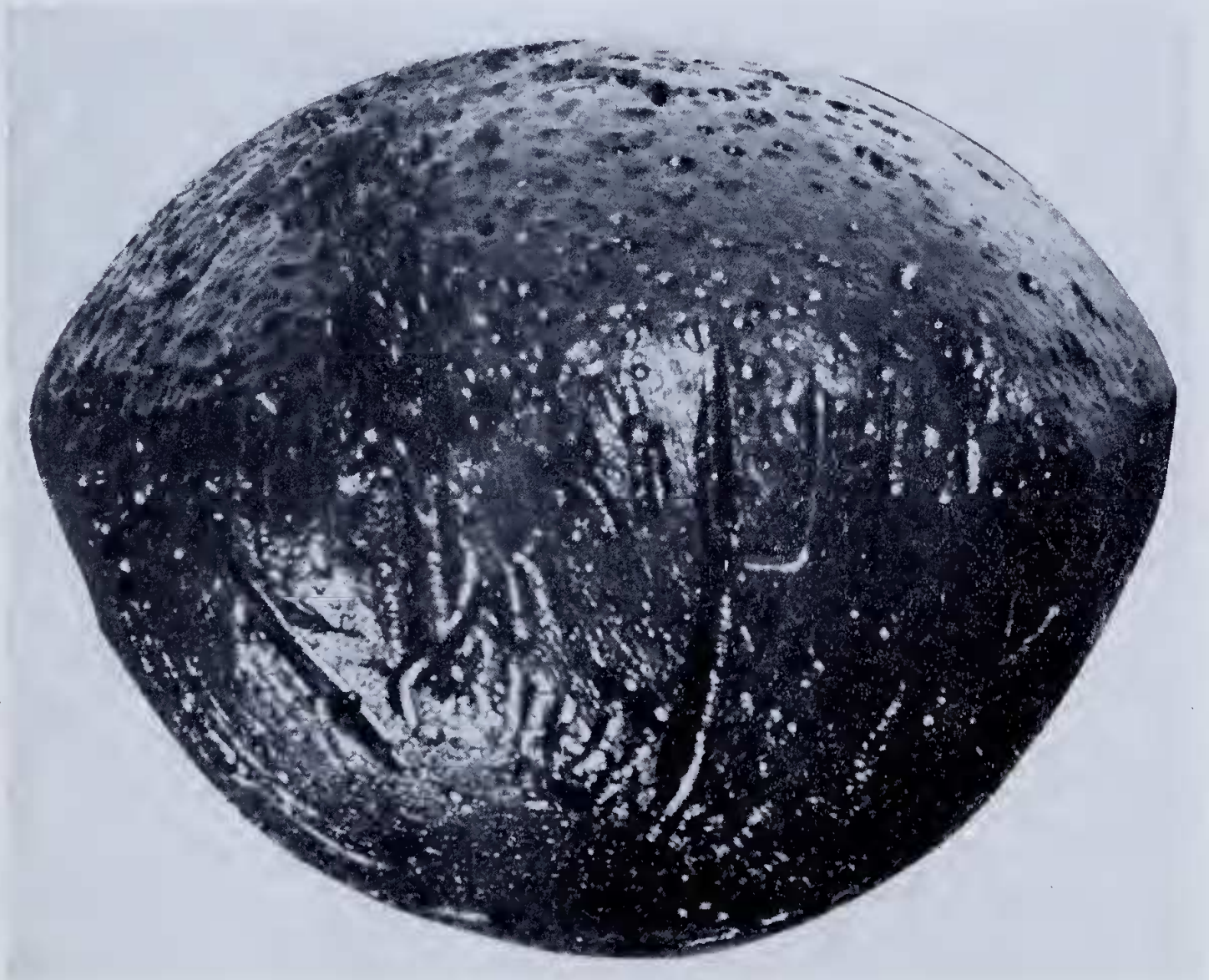
Figure 2.—Sculpture of largest known dumbbell-shaped australite, Cuballing, Western Australia. x3.45 Enlarged end-on aspect of larger gibbosity, showing pits and gutters. Some of the gutters intersect at different levels, some are oblique to the flow line trends of the tektite glass. (Photograph by R. K. Blair).
